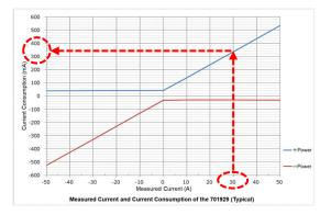
Example: For the 701929, the current consumption at the measured current of 30 [A] is 340 [mA].
